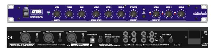
The ART Model 416 Six Channel Personal Mixer quickly and easily combines six sources – three microphones (or balanced line inputs) and three stereo line inputs into a single stereo line-level mix. It has effects patching and phantom power (included to activate condenser microphones or active DI boxes).
